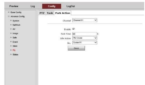
The screenshot shows the 'Park Action' configuration page in a web interface. The 'Park Action' tab is selected. The 'Channel' dropdown is set to 'Channel 01'. There is an 'Enable' checkbox, a 'Park Time' input field with '60', an 'Idle Action' dropdown set to 'PE Cruise', and an 'No.' dropdown set to 'Circle 01'. A 'Save' button is located at the bottom.
