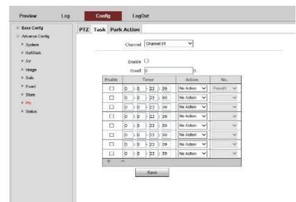
The screenshot shows the 'Task' configuration page in a web interface. The 'Park Action' tab is selected. The configuration includes an 'Enable' checkbox, a 'Dwell' input field with '0', and a table for defining task actions.
