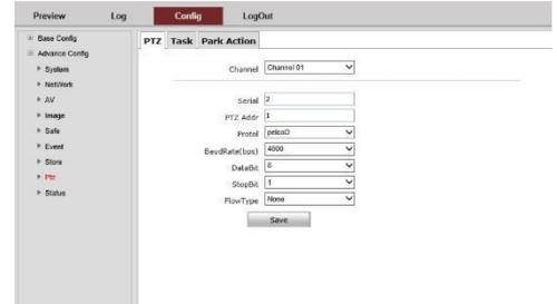
The screenshot shows the 'PTZ Task' configuration page in a web interface. The 'Park Action' tab is selected. The configuration includes a 'Channel' dropdown set to 'Channel 01', a 'Serial' input field with '2', a 'PTZ Addr' input field with '1', a 'Protocol' dropdown set to 'PelcoD', an 'EbusRepeat (bps)' dropdown set to '4800', a 'Default' dropdown set to '8', a 'StopBk' dropdown set to '1', and a 'FlowType' dropdown set to 'None'. A 'Save' button is located at the bottom.
